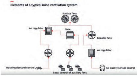
The increased number of sensors around mine sites and the improvement in network connectivity can boost a VoD system's accuracy ABB says
