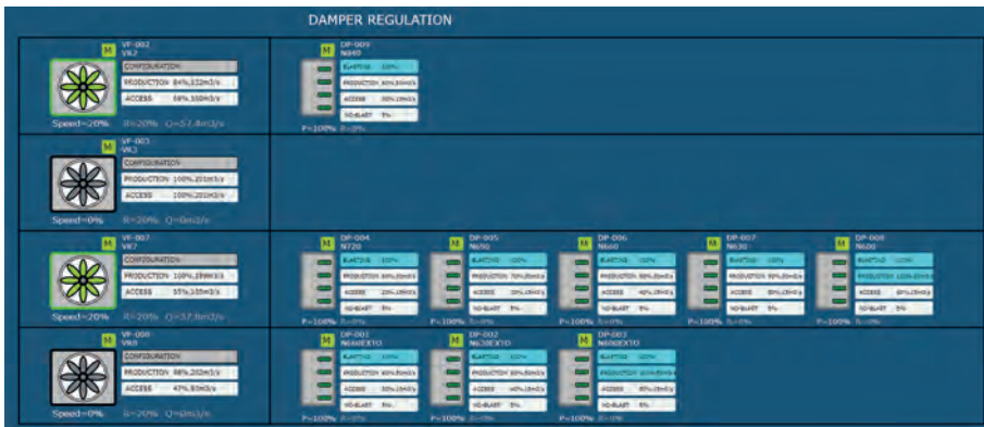
The Zitrón monitoring system: The control panel showing the ventilation system, above, and a representation of the control system of the main equipment, dampers as a function of the ventilation requirements at each production level, below. Both taken from a mine in southern Europe
